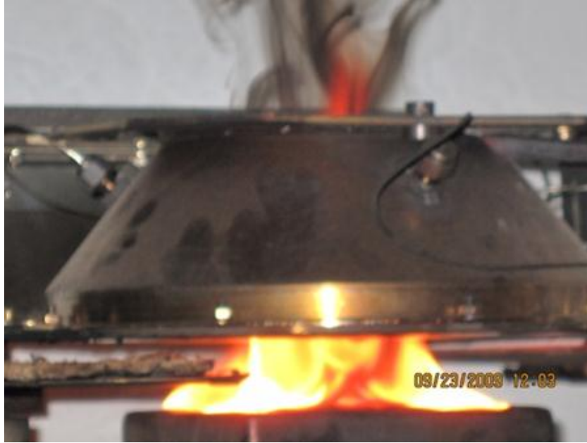
Figure 4.2: Cone calorimeter test with E-glass/polyester
