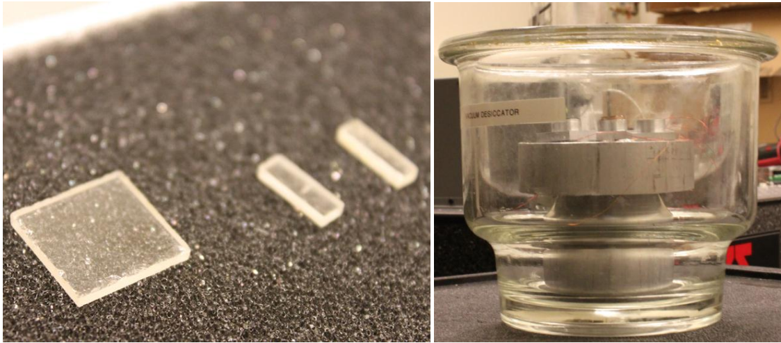
FIGURE 2-4: Left: Insulator, Right: Vacuum used for pumping out air in the epoxy.
