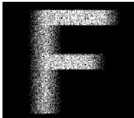
Fig. 4.8. Simulated image for anamorphic lenslet with ROC of 14.6 mm for short (vertically) oriented axis and 15.3 mm for long (horizontally) oriented axis at imaging plane for 14.6 mm ROC.
