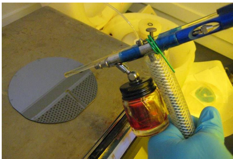
Fig. 5.7. Image of airbrush setup used to generate spray coatings.
