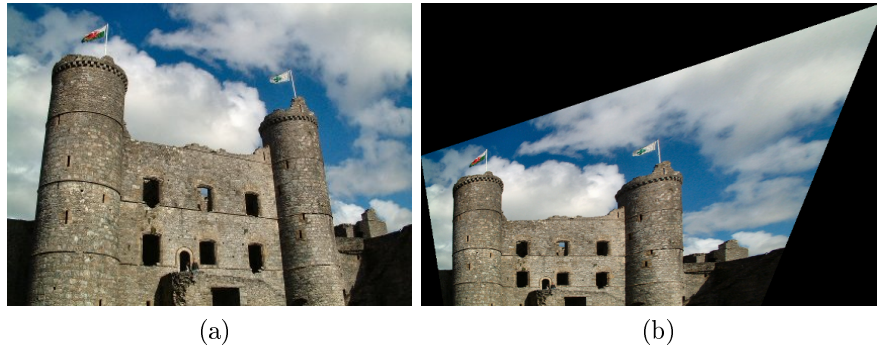
Figure 3.1: Rectification of a façade image taken from an arbitrary pose into an elevation view. (a) is a façade image taken from arbitrary pose. (b) is the automatically converted elevation view image using the method described in section 3.1.1.
