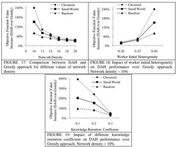
For similar reasons, it is easy to see that the performance advantage of the DAH heuristic would reduce as worker heterogeneity reduces (Figure 18). A similar trend is expected when the knowledge retention rate is high, since it facilitates rapid diffusion of knowledge. This reduces the value of learning from co-workers as well as benefit of waiting to make an assignment (Figure 19).
