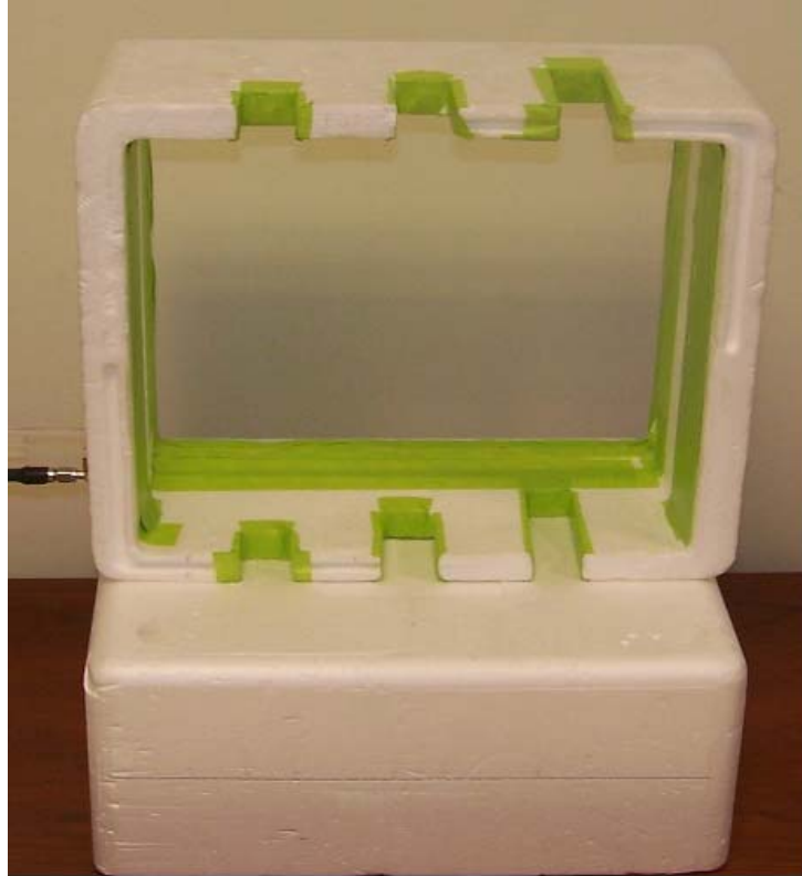
FIGURE 112: Styrofoam structure designed to hold S models in place for test
