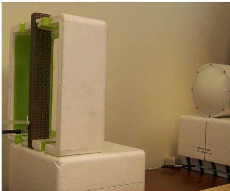
FIGURE 116: Test setup with 4S model and the plane wave transmitter on right
