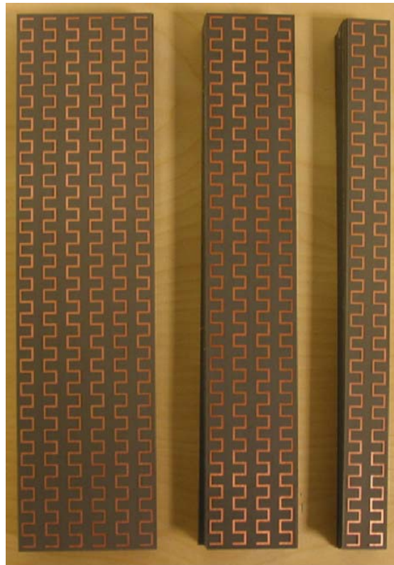
FIGURE 111: Three S models, referred to as 6S, 4S and 2S respectively
