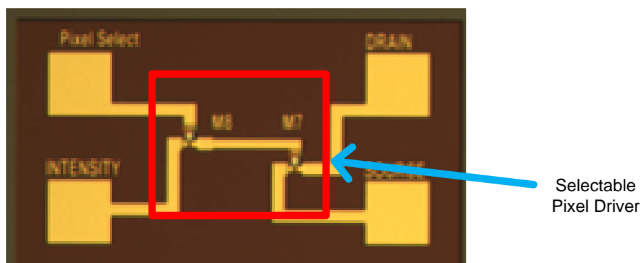
Figure 4.12. Photomicrograph of fabricated selectable ZnO thin-film FET pixel driver circuit.
