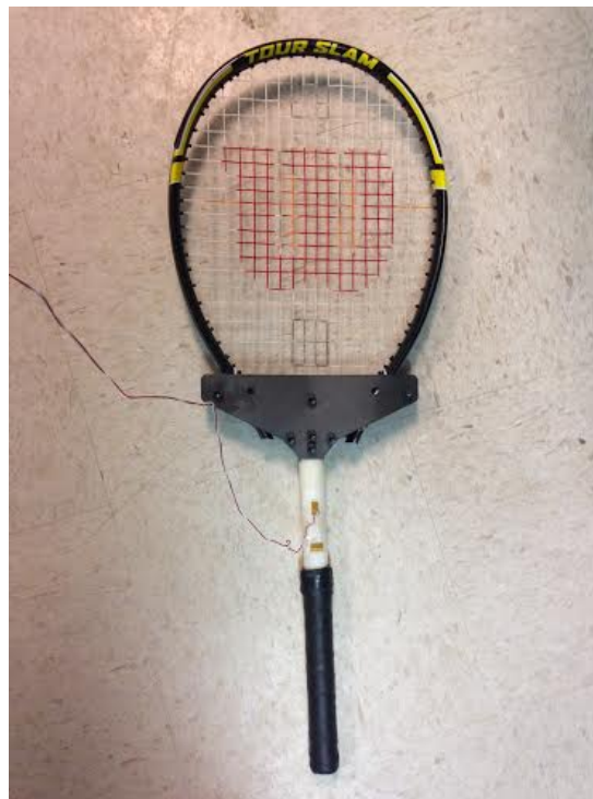
Figure 3.13: New instrumented tennis racket
