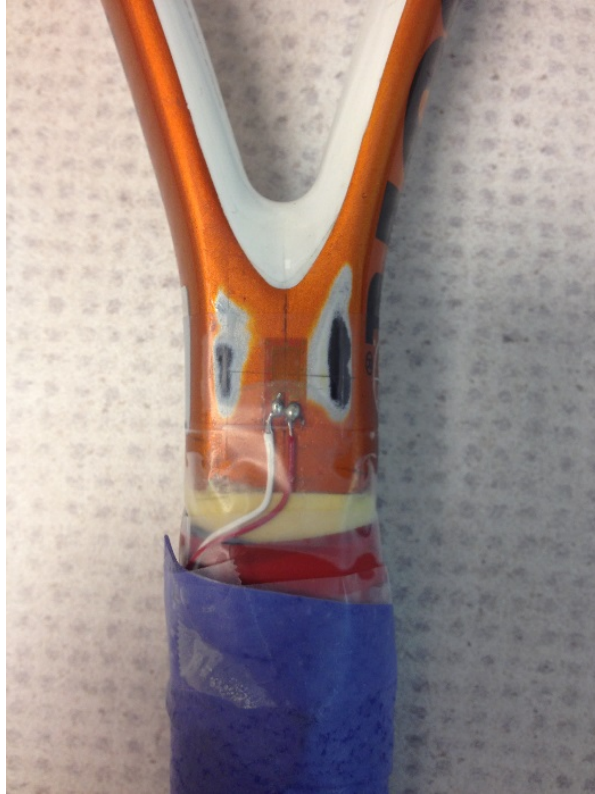
Figure 3.1: Strain gauge attached to the racket
