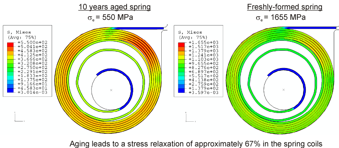
FIGURE 4.5: Comparison of the von-Mises stress profile of the torsional spring- aged for 10 years (left) to that of a freshly-formed spring
