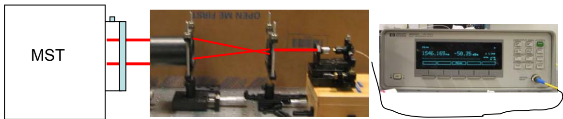
Figure 3- 11 : Wavelengths measured (using a wavemeter) in the MST during a measurement
