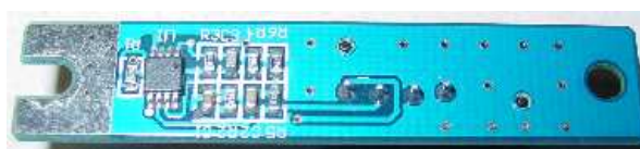
Figure 49d. The final TDS PCB. The PCB layout changed due to avoid high failure rate when IR reflow soldering. The PCB color was changed to avoid confusion with the previous version.
