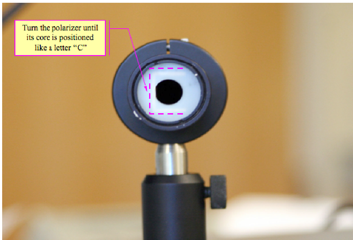
Figure 67: Core of the polarizer #17 positioned like a letter "C".
