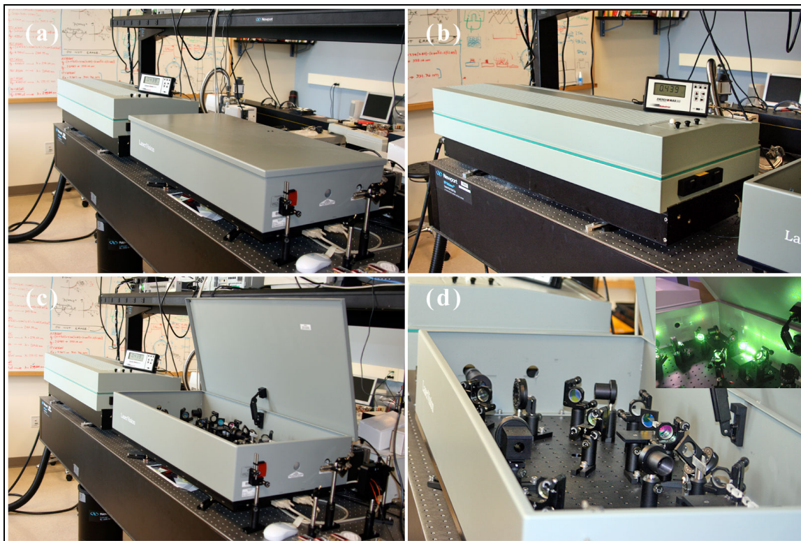
Figure 91: (a) Q-switched Nd:YAG laser (Powerlite ® 8000, Continuum) used to pump an (b) Optical Parametric Oscillator/Optical Parametric Amplifier (OPO/OPA) system (LaserVision, Bellevue, WA), whose details are shown in (c) and (d).
