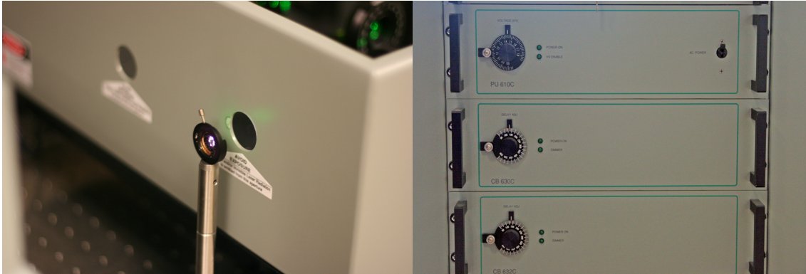
Figure 44: Delay adjustment knob of the YAG's capacitor bank CB 630C (right), and the adjustable iris placed at the input of the OPO/OPA system to reduce the size of the laser beam (left).
