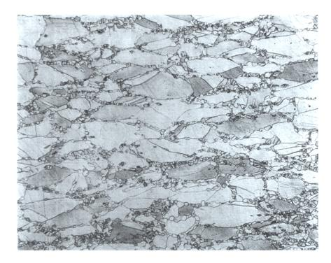
FIGURE 4.1: Microstructure on the surface of an as-rolled billet showing 'necklace' structure (Courtesy: ATI Allvac).
