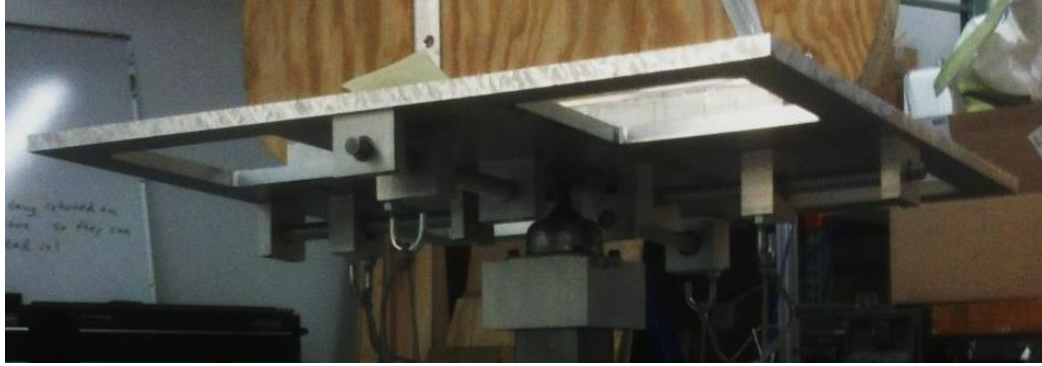
Figure 2.12: View of the ball joint installed between the adapter and pivot plate.
