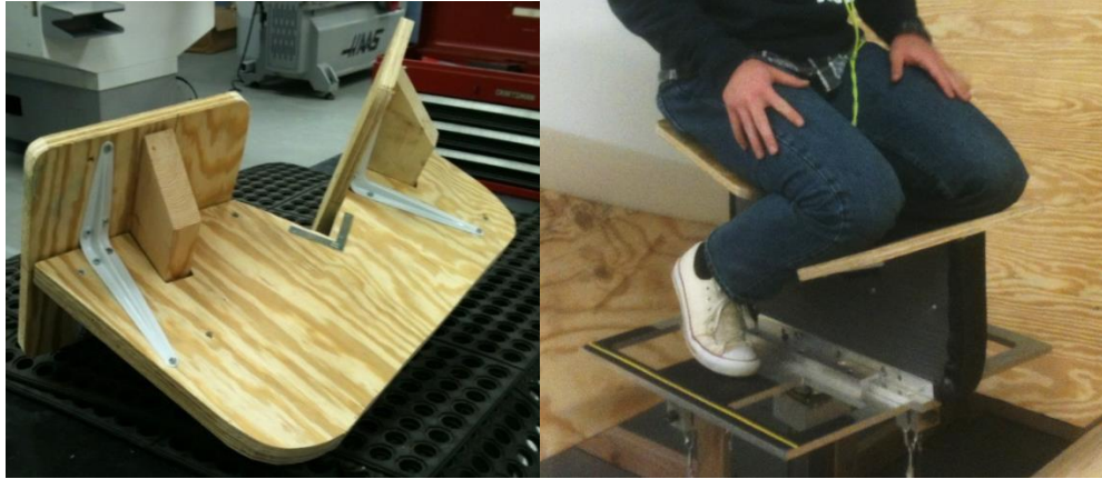
Figure 2.8: Basic wood components of kneeling chair (left), incomplete kneeling chair being tested (right)
