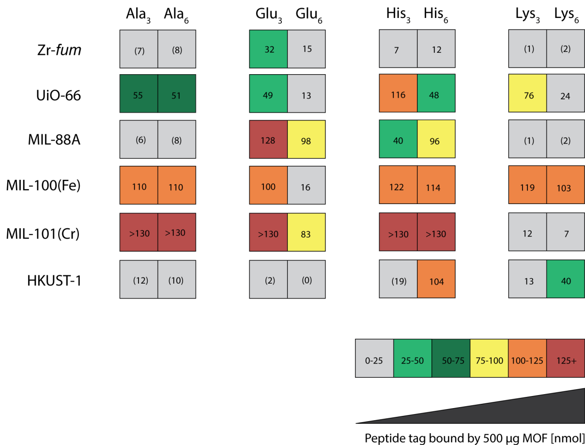
Figure 42 Heat map summary of experimentally determined peptide tag binding capacities. The average binding capacity in nmol observed for 500 \mu g MOF was rounded to a full number and denoted within the center of each box. A number in brackets indicates the absence of a linear relationship between the amount of offered MOF and the amount of respective peptide tag bound by it as determined by low R^2 values observed for linear regression. Each column represents a tripeptide/hexapeptide tag pair, from left to right: Ala, Glu, His, Lys. Each row depicts one of the screened MOFs, from top to bottom: Zr-based Zr- fum and UiO-66, Fe-based MIL-88A and MIL-100(Fe), Cr-based MIL-101(Cr), Cu-based HKUST-1. Boxes were color-coded according to determined tag binding capacities; gray and light green illustrate low (below 50 nmol), dark green and yellow intermediate (50-100 nmol), orange and red high (above 100 nmol) observed binding capacities.
