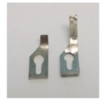
Figure 18. Improvement of the head-fixation bar. Improved holder (on the right) has a longer head-attached bar that provides stronger hold for the head-fixation.
