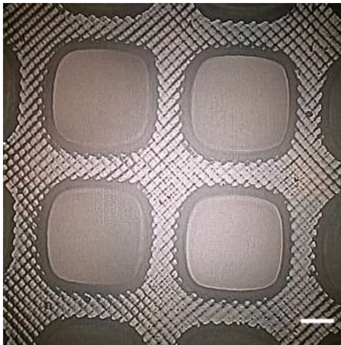
Figure S2. Representative optical image of the surface of the as-printed hydrogel structure, regardless of n_{\text{PEGda}} value. The diamond array can be clearly seen throughout the structure. Scale bar, 200 \mu\text{m} .
