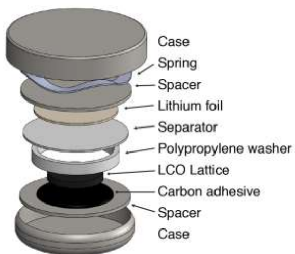
Figure S5. Schematic of the coin cell stack in the 2032 size coin cells.
