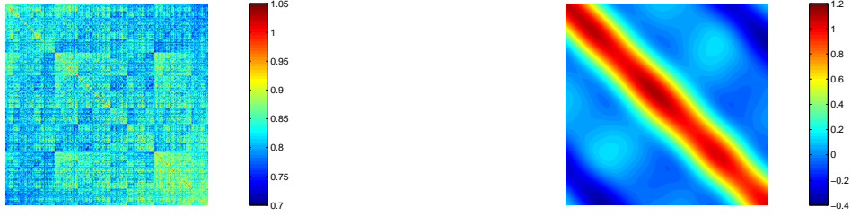
Figure 6: Gram matrices of images of sparse vectors (left) and low-rank matrices (right).
