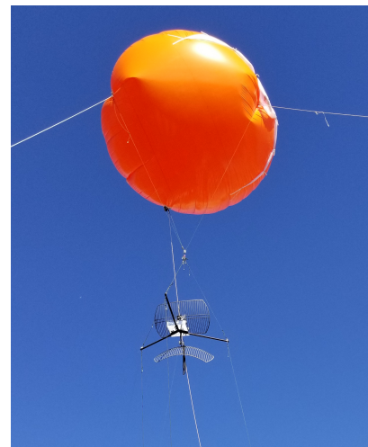
Figure 8. Payload and aerostat during flight test.
