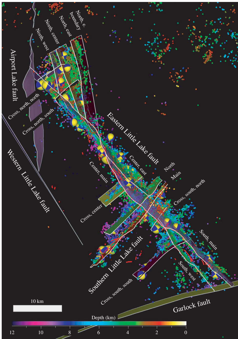
Figure 9. Map view of the final model of the 2019 Ridgecrest faults, including the ELLF and SLLF zones (colored surfaces).
