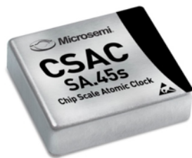
Figure 2-11: The Chip Scale Atomic Clock (CSAC): A RF Frequency Reference for the comb repetition rate stabilization will be needed where no GPS signal is available.
