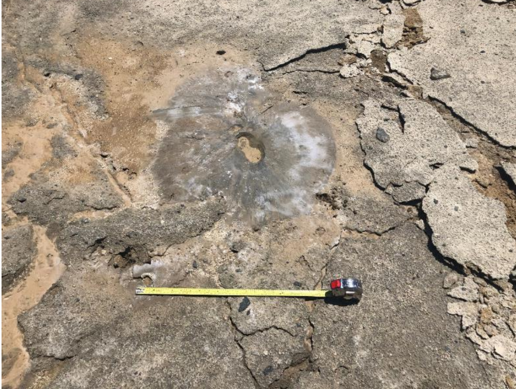
Figure S12. Sand boils within the Salt Wells Valley on 7/12/2019. Area has small sand boils and lateral spread features, located along the M 6.5 surface rupture. Extent of sand ejecta approximately 50 cm diameter. Lat. 35.661949°, Lon. -117.520229°. Photo 6795 credit T. Dawson, CGS.
