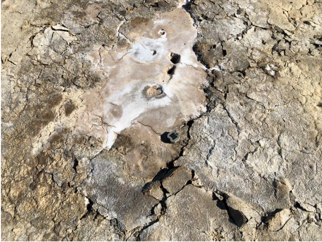
Figure S2. Sand boil in the Paxton Ranch area on 7/10/2019. Lat. 35.807216°, Lon. -117.642838°. Photo 8320 credit B. Olson, CGS.
