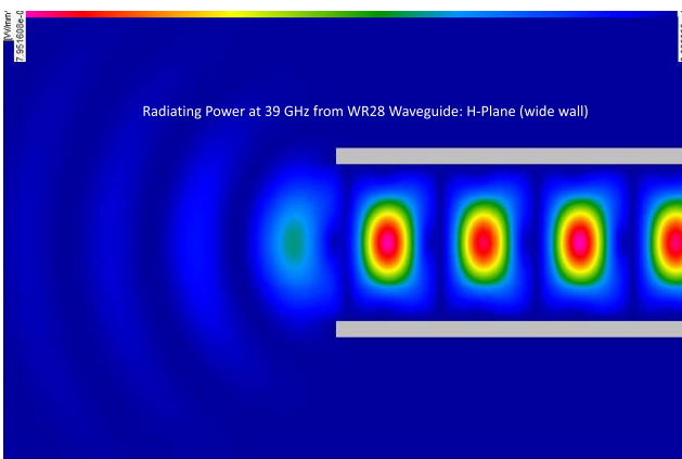
FIGURE 16. Power distribution in the WR-28 waveguide at 39 GHz looking down on the wide wall. Cross section at the center of the vertical wall.
