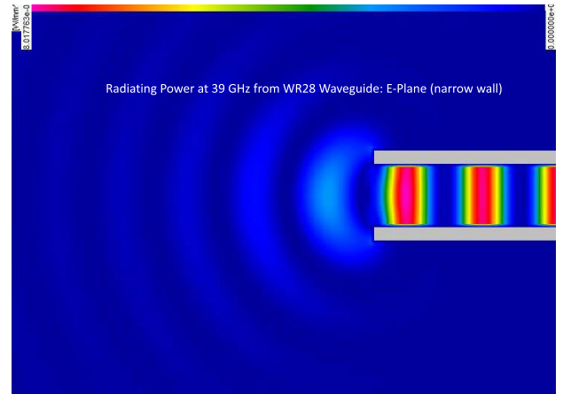
FIGURE 17. Power distribution in the WR-28 waveguide at 39 GHz looking down on the narrow wall. Cross section at the center of the horizontal wall.
