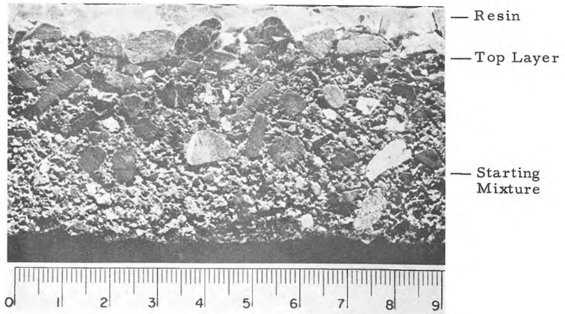
Photograph 1: Armored bed in cross-section, starting mixture II; the section was obtained with the help of resin
