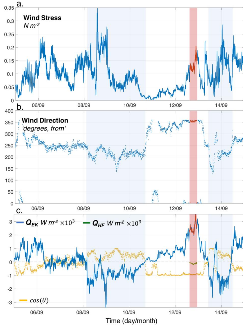
Figure S2: Meteorological measurements made aboard the R/V Investigator during 5 Sep to 15 Sep, 2017. The red band denotes the in-situ sampling period across the front. The blue bands denote periods when the wind is down-front leading to a destabilizing Q_{EK} value. (a) Wind stress; (b) wind direction; and (c) the total heat flux ( Q_{HF} ) during the in-situ sampling (red band), and Ekman equivalent heat flux ( Q_{EK} ) computed assuming a maximum density gradient of M^2 = 1 \times 10^{-6} \text{ s}^{-2} and a fixed orientation for the front (since we only sampled the front at one time, to quantify the effects of preceding and subsequent wind forcing, we take the maximum measured M^2 at the front for the calculation of Q_{EK} but use the longer wind timeseries measured by the ship; this provides us with a proxy Q_{EK} at the front over a period of days rather than hours. This metric assumes the front orientation and gradient remains stationary, so results are more qualitative than quantitative. However, this assumption is reasonable considering the front is a semi-persistent feature over a period of weeks, with similar cross-front temperature gradient, as shown by satellite imagery (Figure 9 of the paper). The resulting Q_{EK} timeseries reveals the wind was strongly destabilizing (reaching -3000 \text{ W m}^{-2} ) for several days up until 2 days before the observations). Yellow circles represent the value of \cos(\theta) : 1 indicates the wind is blowing purely down-front, -1 is purely up-front, 0 is purely cross-front.
