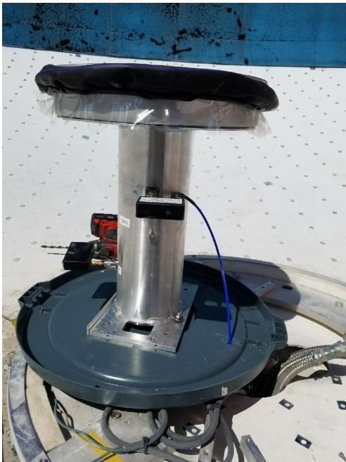
FIG. 3.— The choke-ring feed located at OVRO. It lies in a 6 m dish which is used as a horizon shield. The 6 m dish blocks up to 25^\circ above the horizon. 191 Mpc is \sim 33\% .
