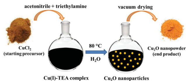
Fig. 1 Schematic representation of the large-scale production of Cu 2 O nanoparticles.
