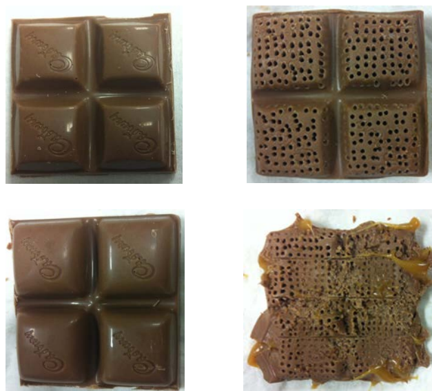
Figure 5-26. Top: The whole milk chocolate bar before and after puncture; Bottom: the Caramello chocolate bar before and after puncture (from left to right).
