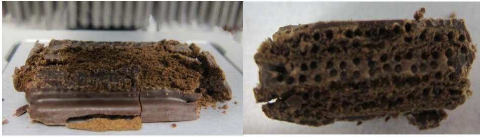
Figure 5-14. The attachment travelled down to puncture the Tim Tam biscuit (a) from the top and (b) through the cross section (sample was cut in half).
