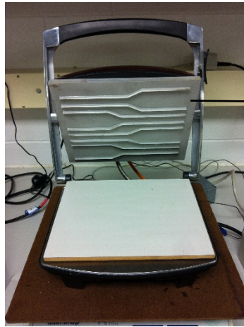
Figure 5-38: The setup of the hot plate press used for the production of the slip extrusion bags.
