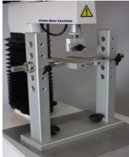
Figure 5-35: The TA-TR Tube Roller Extrusion Fixture ("The squeeze test for tubes and packets," 2014).
