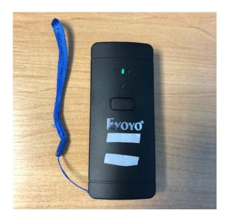
Figure 3.11 Pocket 2-dimensional (2D) barcode scanner.
