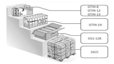
Figure 2.7 Identification in each level of packaging using GS1 standards.
