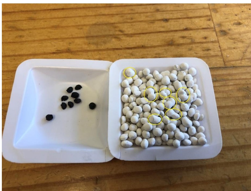
Figure 44. Vortex mixer pelleted onion seeds. The yellow circles indicate the clumps cannot be totally avoided even if stirred with a stirring rod several times.
