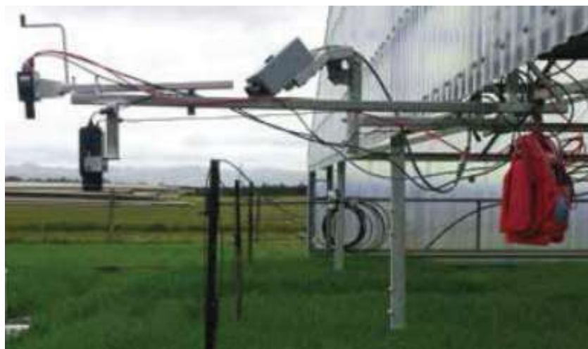
Figure 3-6: Sensors are being trialled to directly monitor plant water stress (Jafari et al. , 2016)
