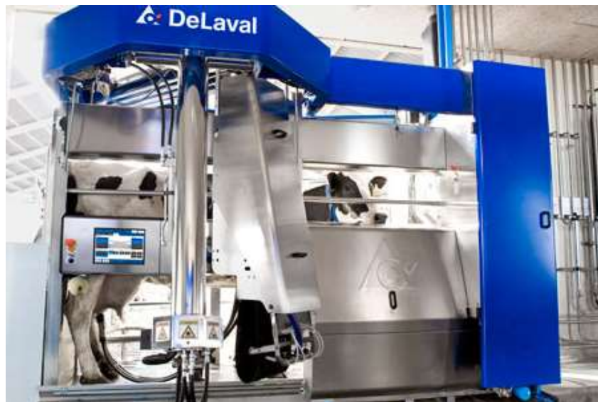
Figure 3-7: An automatic milking robot unit in practice (source: www.DeLaval.com )
