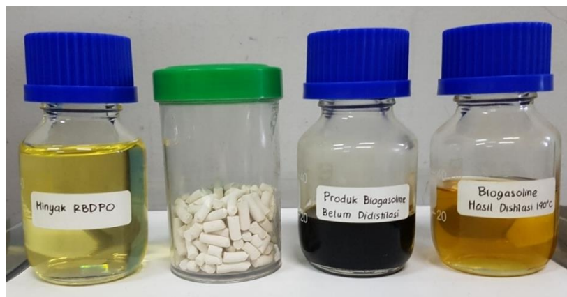
Fig. 5.5 Feedstock (left), catalyst (middle left), and green gasoline products before & after distillation (middle right and right) through hydrodeoxygenation of refined palm oil ( T=450\text{-}550^{\circ}\text{C} ; atmospheric pressure; liquid biohydrocarbon yield=45-53%;). (ITB laboratory, 12 th May 2017)
