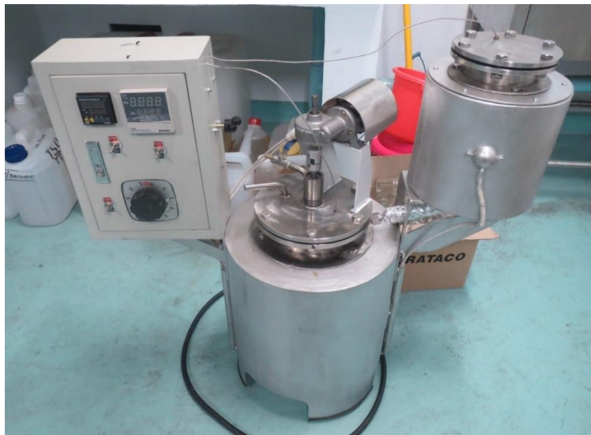
Fig. 5.8. Reactors for liquid biohydrocarbon production from fatty acid: (i) green diesel production through metal soap decarboxylation and (ii) green gasoline production through metal soap pyrolysis (ITB Indonesia, 2015, picture by ITB)
