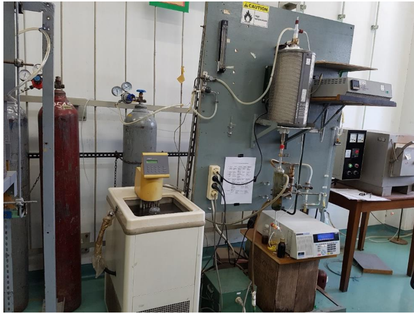
Fig. 5.4 Laboratory scale production of green gasoline from vegetable oil through hydrodeoxygenation (ITB laboratory, 12 th May 2017)
