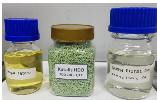
Fig. 5.3 Refined palm oil feedstock (left), catalyst (centre), and green diesel liquid biohydrocarbon production through hydrodeoxygenation (right) (T=450-550°C; atmospheric pressure; liquid biohydrocarbon yield=45-53%). (ITB laboratory, 12 th May 2017)
