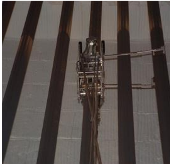
Figure 2-16 MP LEO-SCAN Reformer Tube Inspection system
