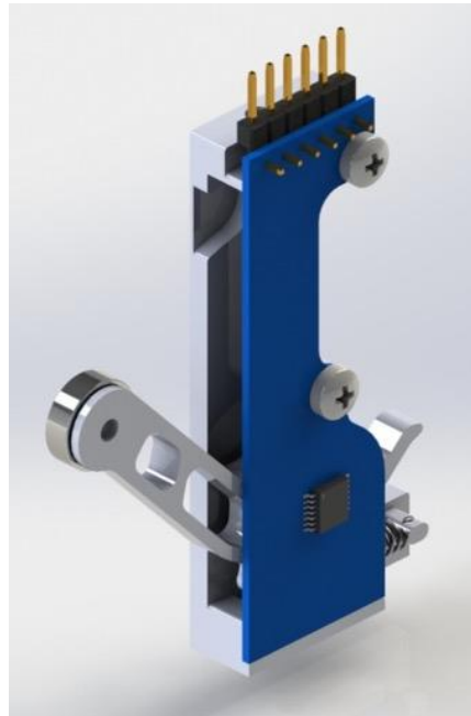
Figure 5-10 Displacement Sensor CAD image in SolidWorks
