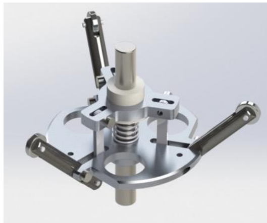
Figure 5-27 TPS design 3D CAD Model
