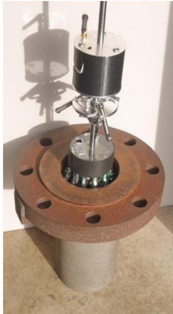
Figure 5-43 Experiment Setup of FTIS system measuring Reformer Tube Sample A
