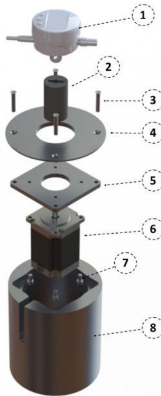
Figure 8-1: Sample Tube Internal Profilometry Analyzer Explode View
