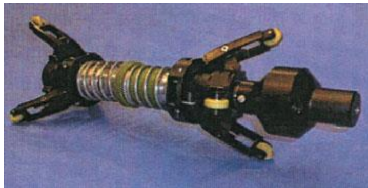
Figure 3-9: Typical LOTIS Laser probe with the Three-point Centralizing mechanism [10]
