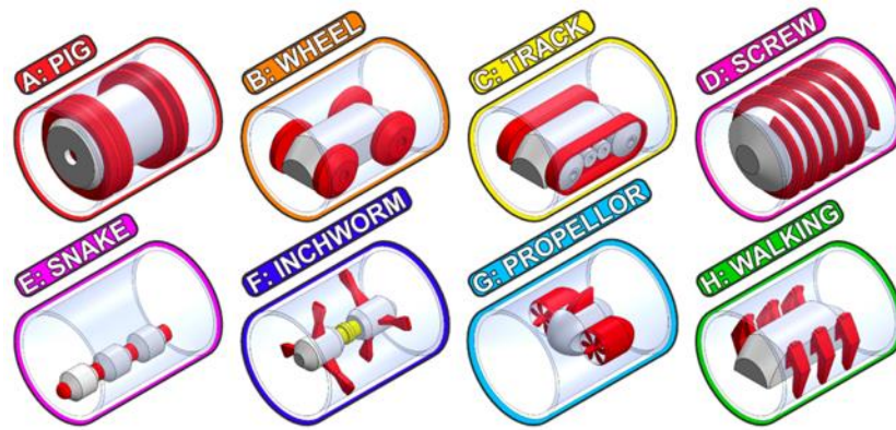
Figure 5-3 Classification of in-pipe robots [117]
