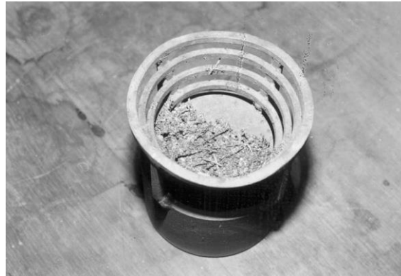
Figure 2-9 Broken pieces of catalyst on the retaining ring [31]
