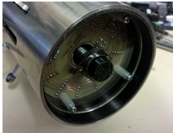
Figure 5-41 Photo of the MaxBotix LV-MaxSonar-EZ4 sensor extruding through the bottom acrylic cover
