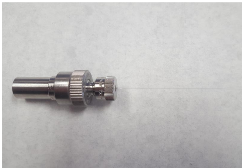
Figure 4.15 Swagelok fittings for connecting capillary to Quantachrome-Autosorb-iQ2.
