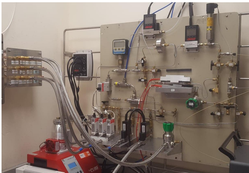
Figure 2.12 A photo of our breakthrough test apparatus (It should be noted that the upper part of the apparatus is used for the measurement of membrane permeability).
