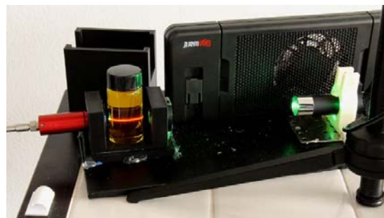
Figure 4. Partial view of the Raman Probe. Parts 5 – 7 in figure 3 are inside the red cylinder
