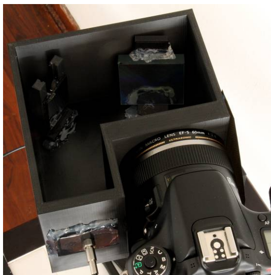
Figure 2. Internal view of the spectrometer, showing the simple optical bench
