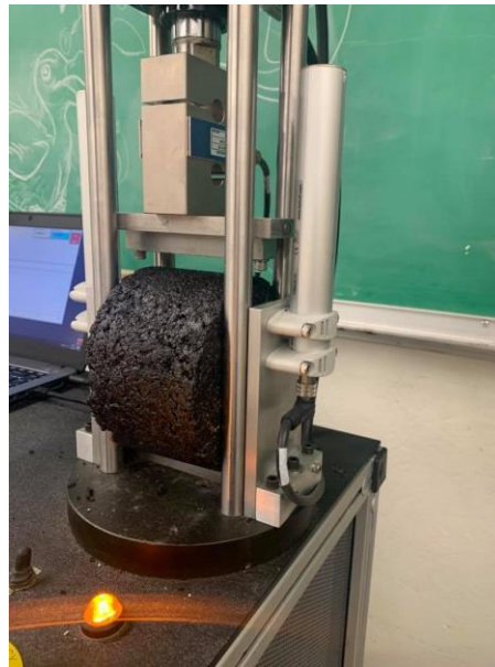
Figure 17: Indirect Tension Test Fixture
