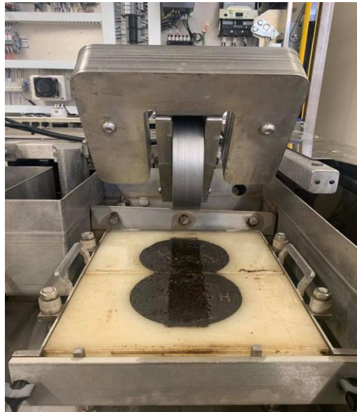
Figure 20: Samples in the HWTT Fixture
