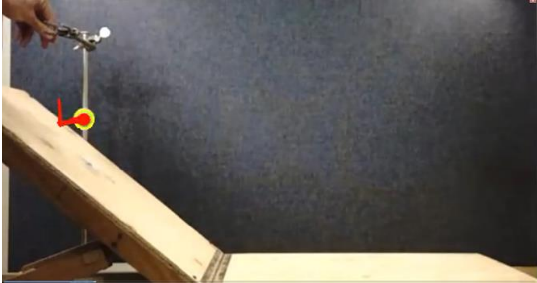
Figure 4-3 Object tracking sample using OpenCV. The ball color is used to track the object and the trajectory is superposed.
