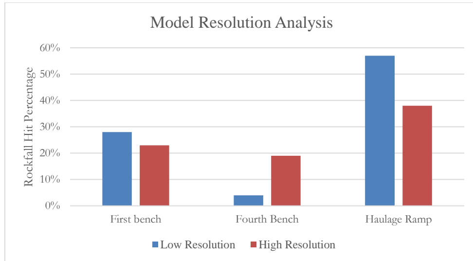
Figure 5-8 Comparison between the outcome for the low and high resolution of the input terrain model.
