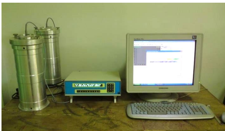
Fig. 3 - Test setup for the hydration heat test.
