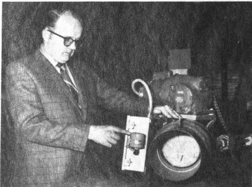
Figure 15. Vander points out the vertically mounted pressure sensor. The downstream end of the valve assembly is also pictured.
