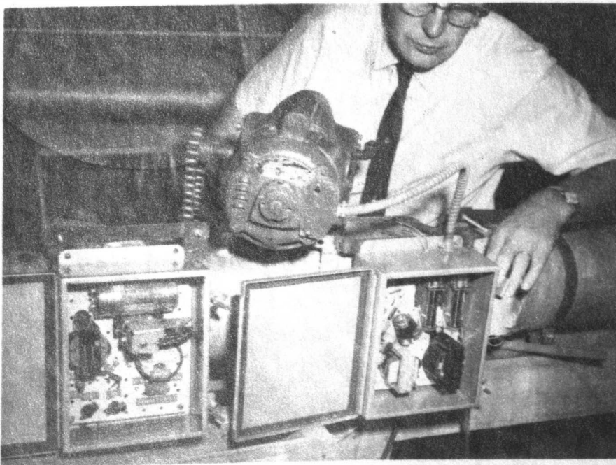
Figure 16. Dr. Wierma is pictured with the Program Control on the left and the valve control on the right.
