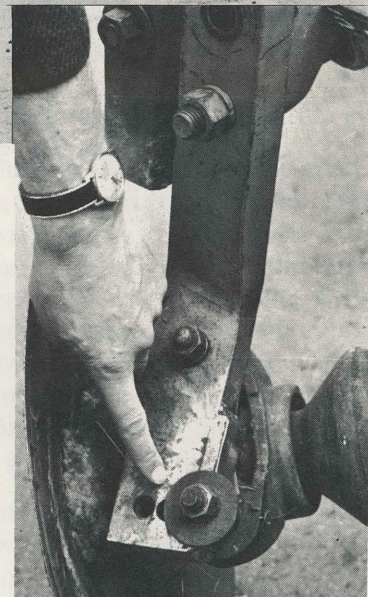
Figure 11. Mountings for disks should be flexible enough to allow disks to ride over rocks and similar obstacles. Disks can be mounted so that they "break-away" when they contact a solid obstacle (see insert at right).
