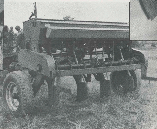
Figure 6b. Corn cultivator shovels with wings welded on either side make suitable furrows for most interseeding in native or bluegrass sods. Weld a supply beforehand. If wings break off, merely change shovels and continue. May be mounted on drill shown above right.
