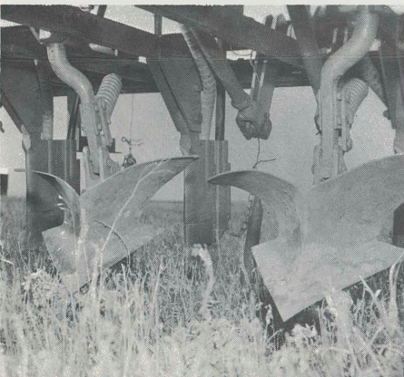
Figure 6a. Sweeps mounted ahead of seeding spout to remove wide strip of sod before seeding slow developing native grasses. May be mounted on drill shown above left.
