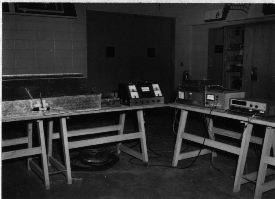
Figure 6. Model of Beef Confinement Building and Monitoring Instruments. From Left to Right: Model, Anemometer (Wind Velocity), Voltage Transformer, Dewpoint Temperature Recorder and Selector Switch (Above), Hotwire Anemometer (Outlet Velocity) and Digital Voltmeter (Output of Hotwire Probe)
