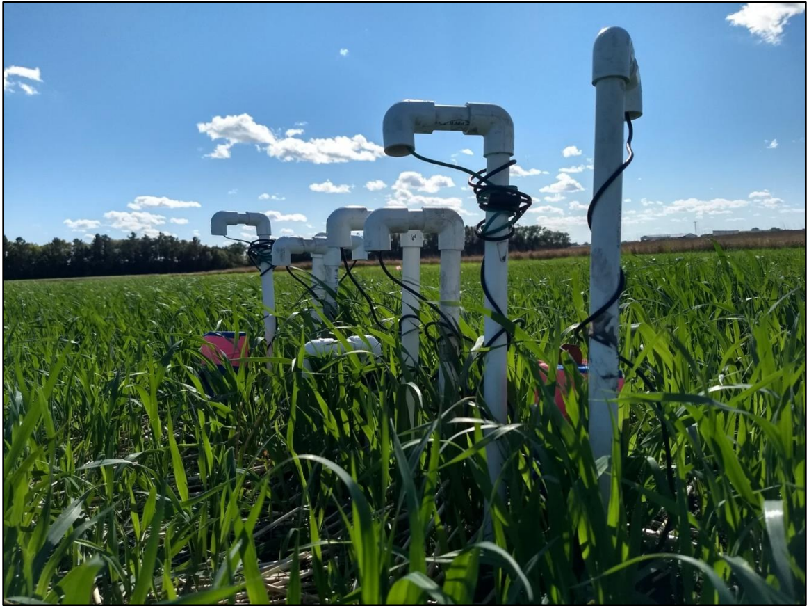
A4.5. Soil moisture, tension and temperature sensors installed at different depths in the field.
