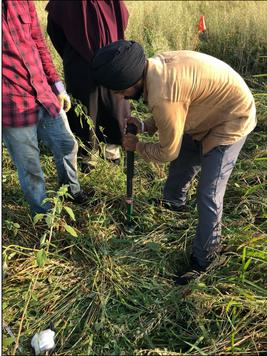
A4.1. Taking core samples from field to analyze soil physical and hydrological properties.
