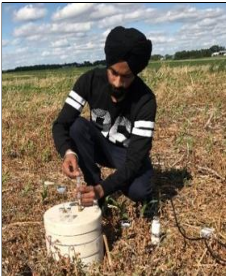
A4.4. Taking gas samples from field to analyze CO 2 , N 2 O and CH 4 emissions.
