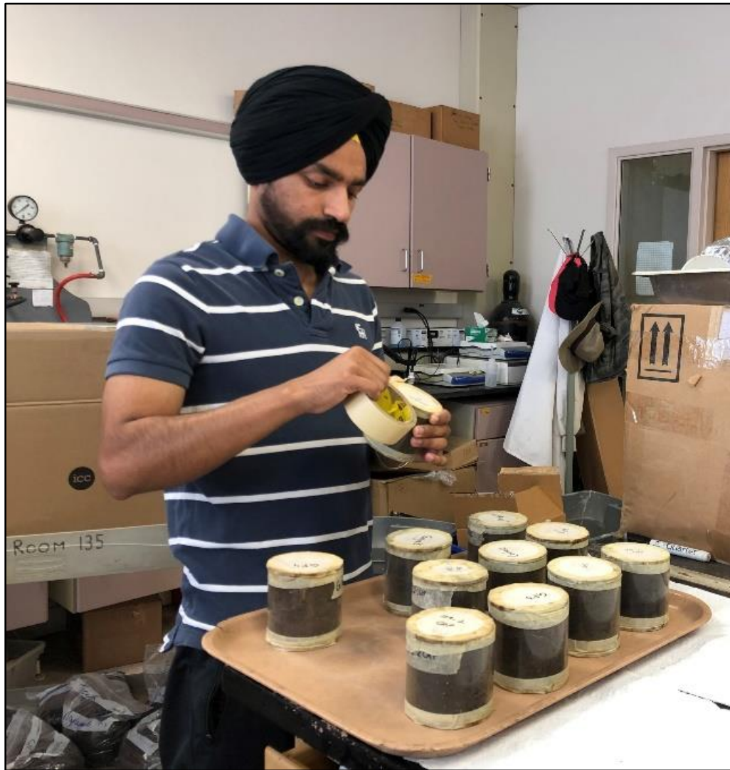
A4.2. Preparing plexiglass cores for computed tomography scanning.
