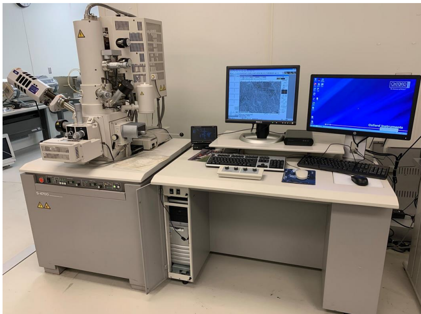
Figure 3.13 Hitachi S-4700 scanning electron microscope.
