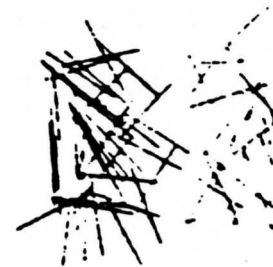
STRAIGHT, SMOOTH DRAWN WIRE FIBERS
