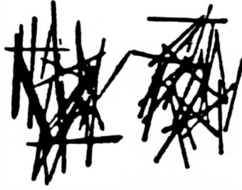
IRREGULAR SHAPE, MELT-EXTRACTION FIBERS
