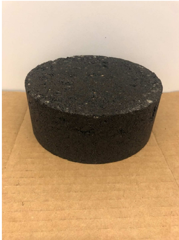
Figure 3.27: Hamburg Wheel Tracking sample after being compacted at a height of 60mm and diameter of 150mm.
