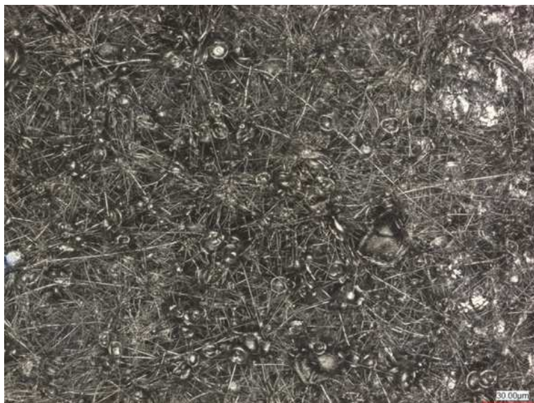
Figure 4.12: LSM Image from Cellulose Nanofibers produced with Solution 2.
