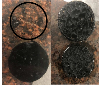
Figure 5.10: Example of adhesive failure (left) and cohesive failure (right) in BBS test.
