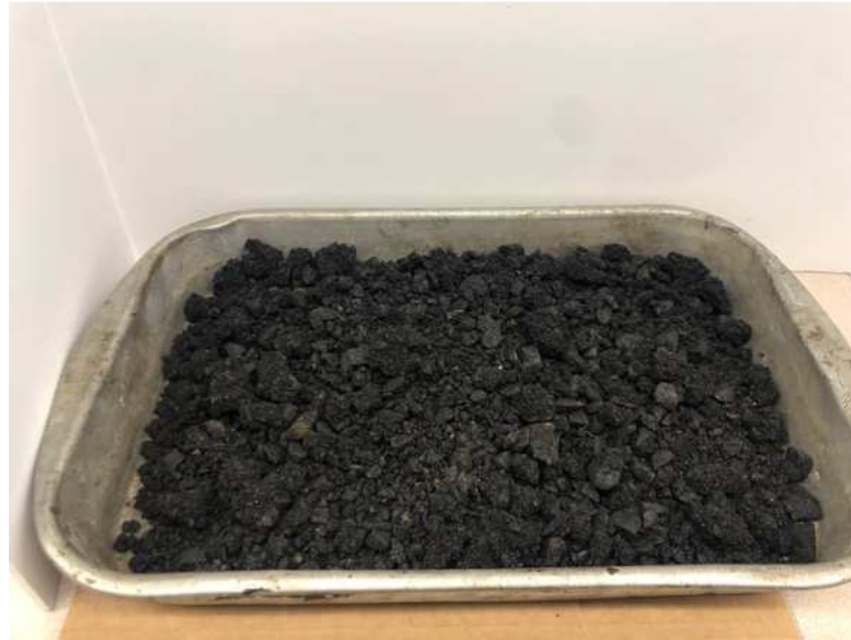
Figure 3.3: Asphalt mix (RAP20) that was collected and used for the study.
