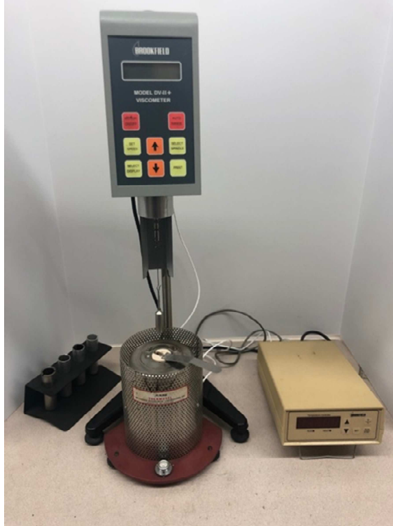
Figure 3.18: Brookfield Rotational Viscometer used for the Rotational Viscometer test.
