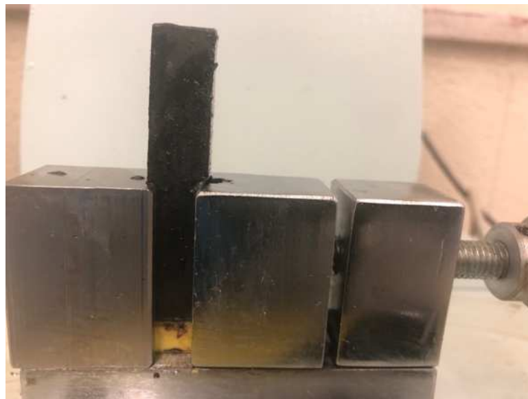
Figure 3.13: Zoom view of the Izod impact strength test sample prior being tested.
