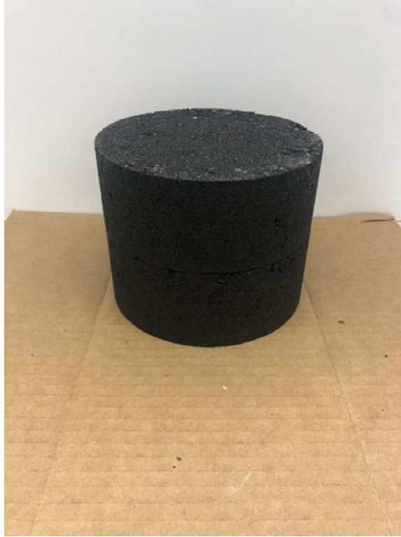
Figure 3.19: SCB sample after being compacted at 150mm diameter and 120mm height
