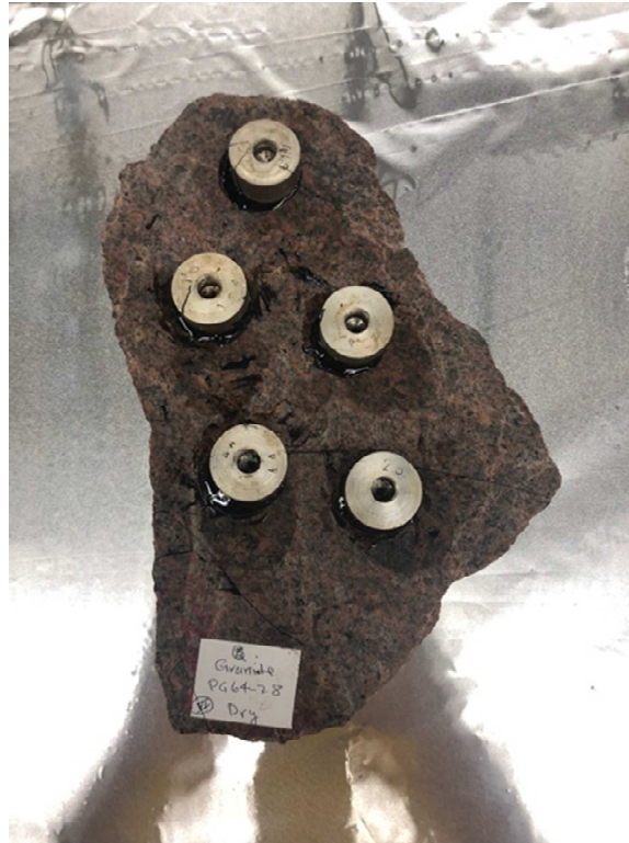
Figure 3.15: View of one aggregate with five samples prior the BBS test.
