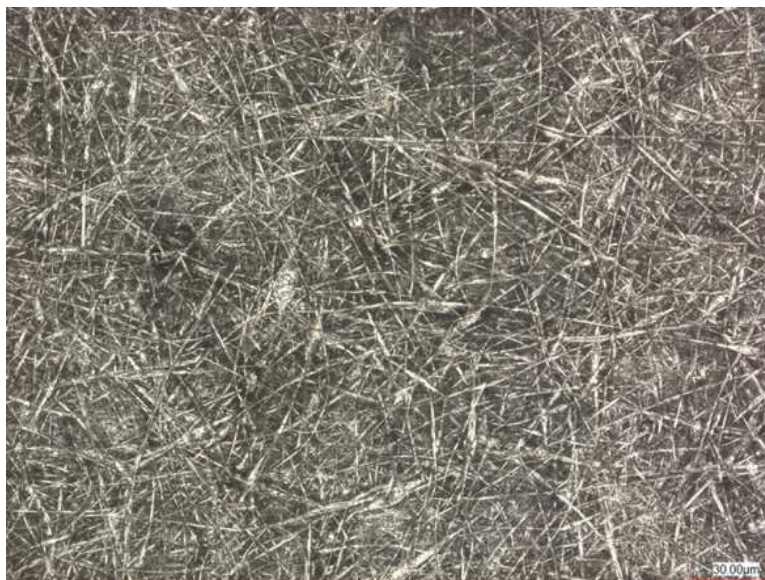
Figure 4.14: LSM Image from Cellulose Nanofibers produced with Solution 4.
