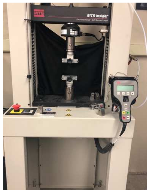
Figure 3.8: MTS Insight 5 Machine used for the CNF Tensile Strength test.
