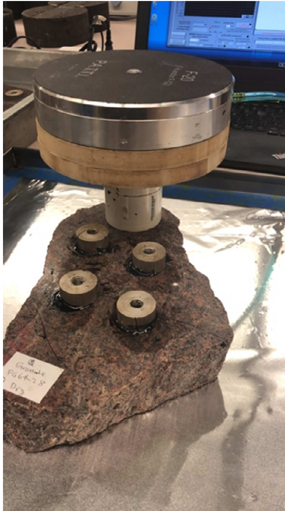
Figure 3.17: View of one of the granites sample being tested using the PATTI machine.
