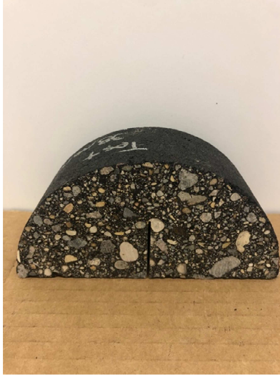
Figure 3.21: SCB sample after the 38mm notch was cut.
