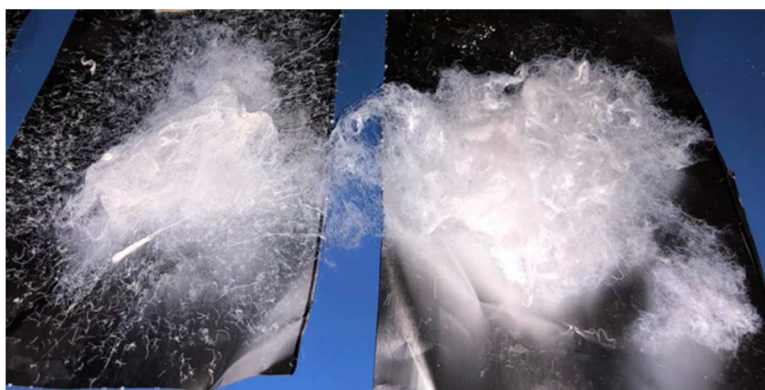
Figure 4.10: Final results of the CNF produced using solution 5 and static electrospinning technique.
