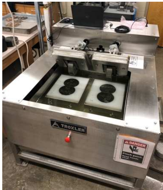
Figure 3.29: Hamburg Wheel Tracking test set up prior testing with the samples in place.
