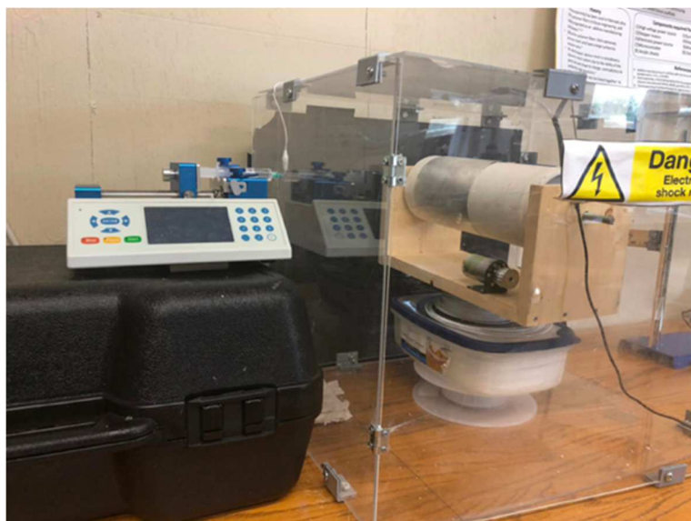
Figure 3.5: Rotating Electrospinning setup used for the fiber production.
