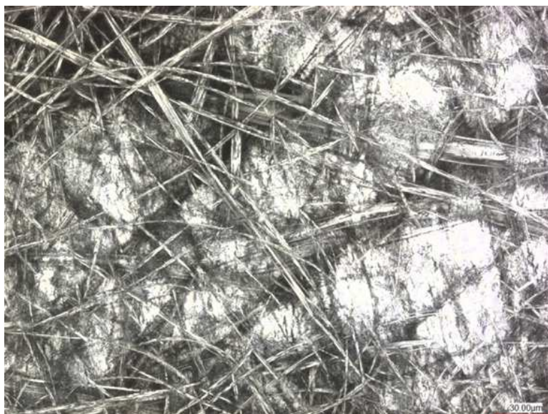
Figure 4.11: LSM Image from Cellulose Nanofibers produced with Solution 1.
