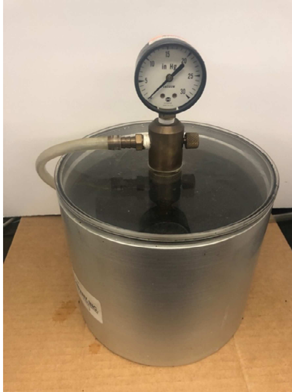
Figure 3.24: TSR sample being Vacuum saturated inside a vacuum chamber.
