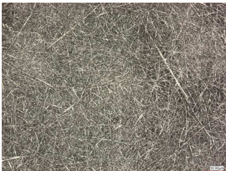
Figure 4.13: LSM Image from Cellulose Nanofibers produced with Solution 3.
