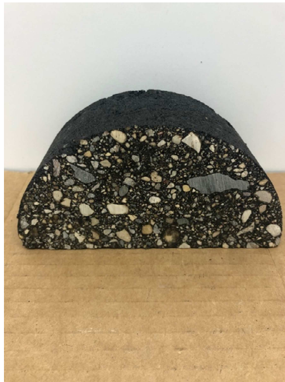
Figure 3.20: SCB sample after being cut into 57mm thickens samples for the SCB test
