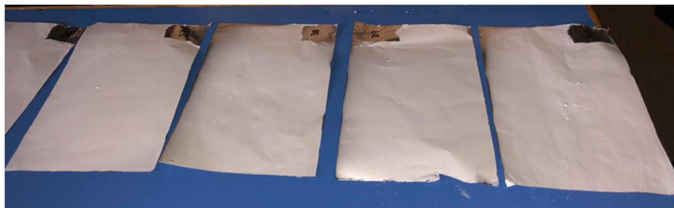
Figure 4.9: Final results of the CNF produced using solution 4 and static electrospinning technique.
