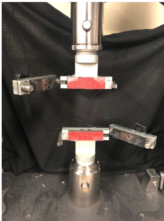
Figure 3.9: Clamp used on the MTS Insight 5 for the Fiber Tensile Strength test.
