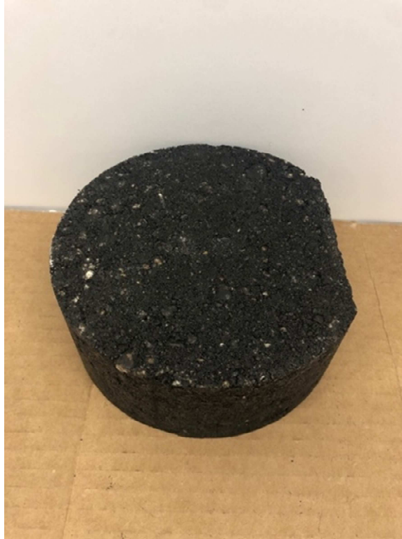
Figure 3.28: Hamburg Wheel tracking sample after being cut to fit in the mold of the HWT testing machine.
