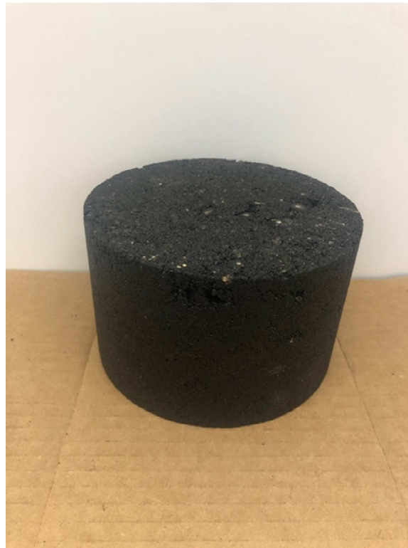
Figure 3.23: TSR sample after it was compacted at a height of 95mm and a diameter of 150mm.
