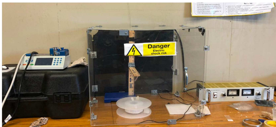
Figure 3.4: Static Electrospinning setup used for the production of the fibers.
