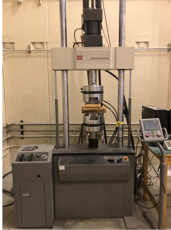
Figure 3.26: MTS ® 810 Material Test System used to conduct the TSR test.
