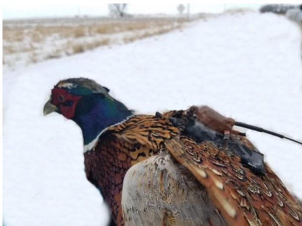
Figure 3-2. Self-made, low-cost GPS tracker weighing 43 g (<5% of body mass) attached to a male ring-necked pheasant in Beadle County, South Dakota, 2019.
