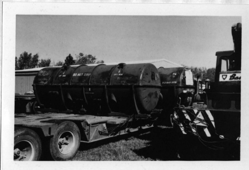
Fig. 14. Canisters containing B-52 bomber engines.
