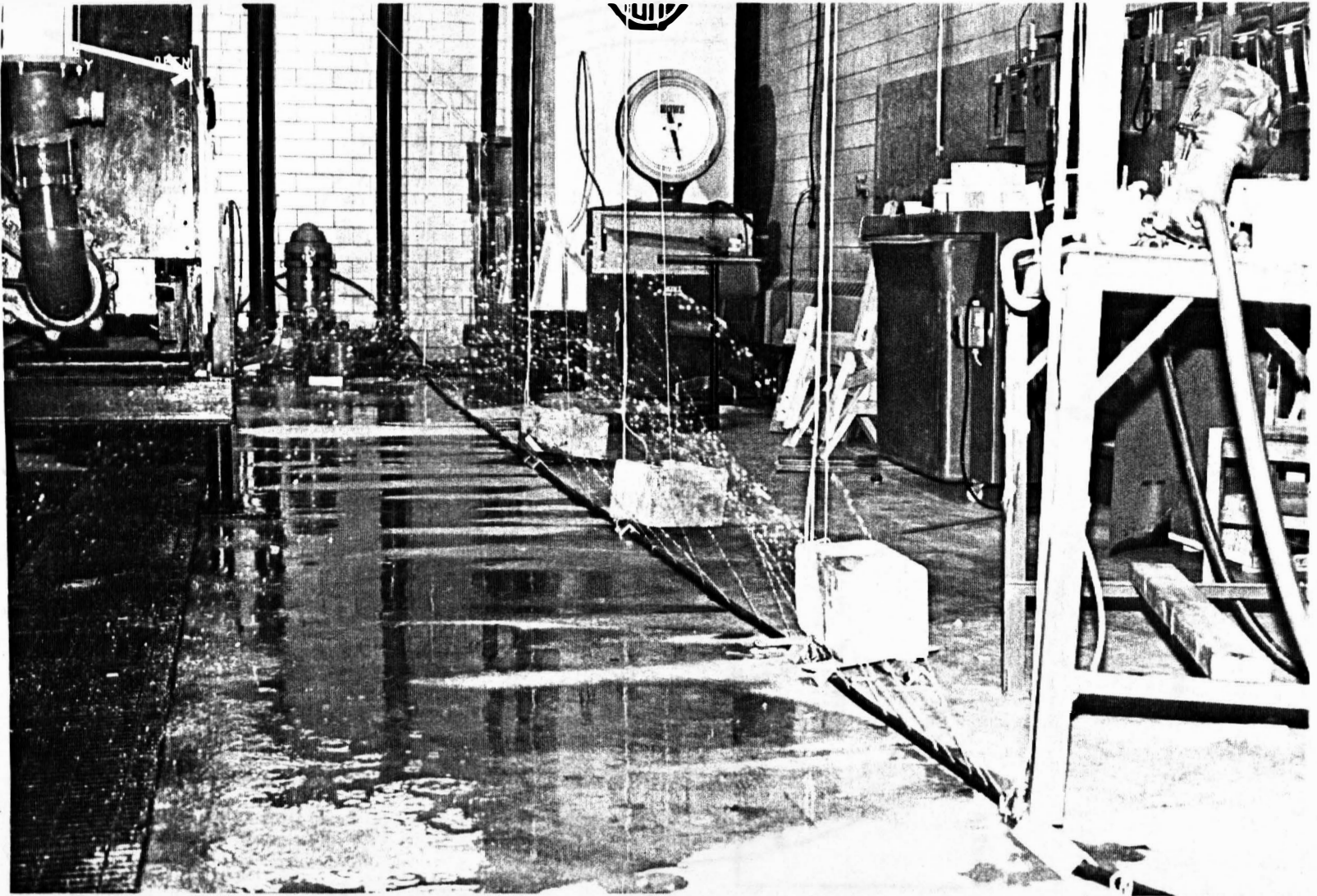
Figure 8: Perforated Poly-Flex and Six Manometers to Measure the Flow Rate and Pressure Distribution
