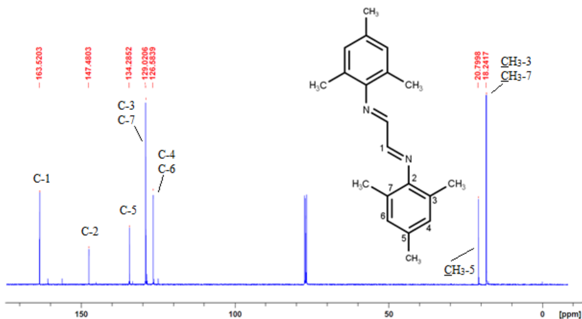
Figura 25: Espectro de RMN ^{13}\text{C} ( \text{CDCl}_3 ; 125,75 MHz) do ligante (2,4,6-Trime).
