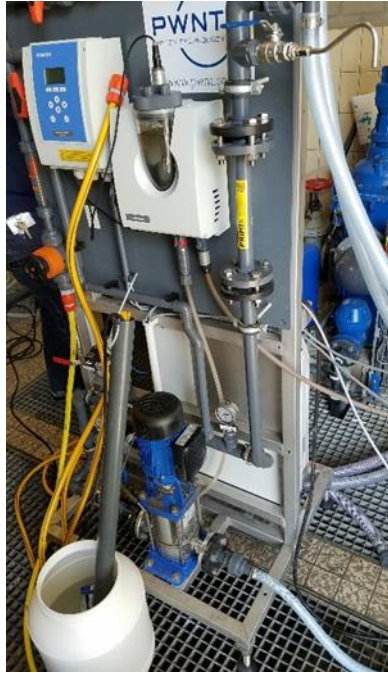
Figure II-1 Pilot Setup for Conductivity Measurements
