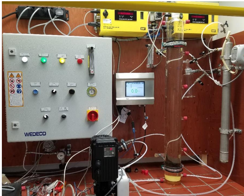
Figure 4-4 Ozone Bench-Scale at HWL in Haarlem
